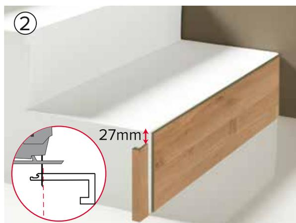
Subsequently, cut the groove at the same measure of the height of the step, subtracting 27 mm. Then clean the groove carefully and stick the plank and the stair nose to the riser using silicone.
