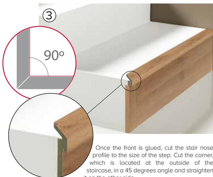
Once the front is glued, cut the stair nose profile to the size of the step. Cut the corner, which is located at the outside of the staircase, in a 45 degrees angle and straighten it on the other side.
